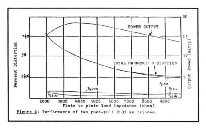
Figure 4 shows the performance of the same tubes connected as triodes. While the power output is substantially reduced, sensitivity to changes in load impedance is also drastically reduced. Power output is still maximized for loads between 3000 and 5000 ohms. If we were to wind the output transformer to reflect 6 ohms as 4000 ohms, we still could not accommodate the entire impedance swing of the speaker.
