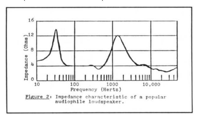
A loudspeaker is far from a constant impedance, and can vary appreciably at different frequencies. Figure 2 shows the impedance vs. frequency curve for a popular high end louspeaker. The manufacturer of this speaker states that is should be considered to be a load impedance of 6 ohms (the nominal impedance), but in fact it presents an impedance that varies from a low of 2.25 ohms to a high of 13 ohms at different frequencies within the audio spectrum.
