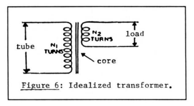
Figure 6 presents a pictoral representation of a transformer and its connections.
